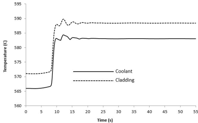
Figure 16. Changes of coolant and cladding temperature after ULOHS accident
