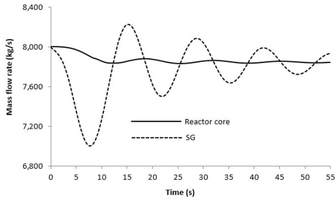
Figure 13. Changes at the coolant mass flow rate and the reactor core SG on ULOHS accident
