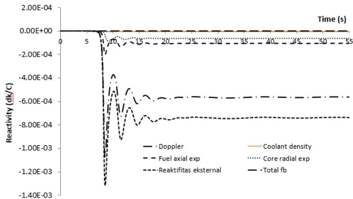
Figure 18. Changes of reactivity for case ULOHS accident
