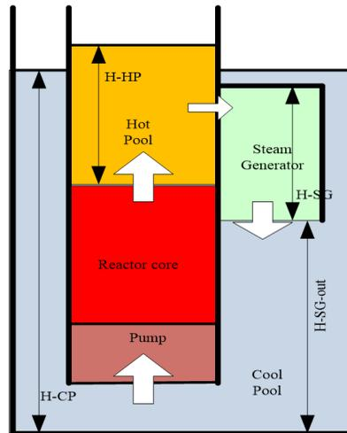
Figure 2. A scheme of coolant flow rate. From “Safety analysis of small long life CANDLE fast reactor”, by Yan and Sekimoto, 2008, *Annals of Nuclear Energy*, 35(5), pp. 813-828. Copyright 2008 by Elsevier
