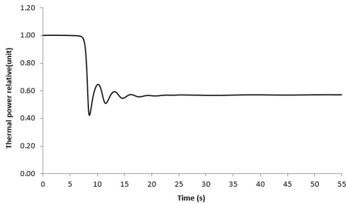
Figure 17. Changes in thermal power after ULOHS accident
